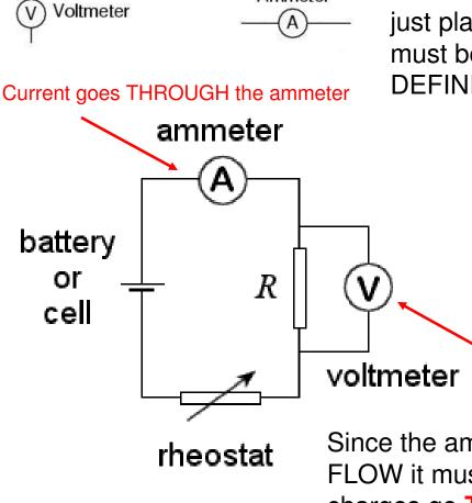
The voltmeter and ammeter cannot be just placed anywhere in the circuit. They must be used according to their DEFINITION.
