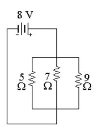
To the left is an example of a parallel circuit. a) What is the total resistance?
