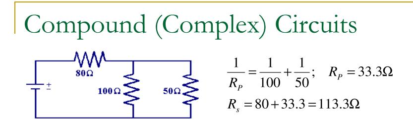
Suppose the potential difference (voltage) is equal to **120V**. What is the total current?
