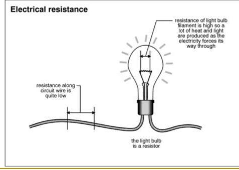
The unit for resistance is the OHM,  $\Omega$
