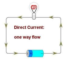
DC = Direct Current - current flows in one direction Example: Battery
