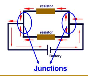
The current going IN to a junction will always equal the current going OUT of a junction. I - I + I + I
