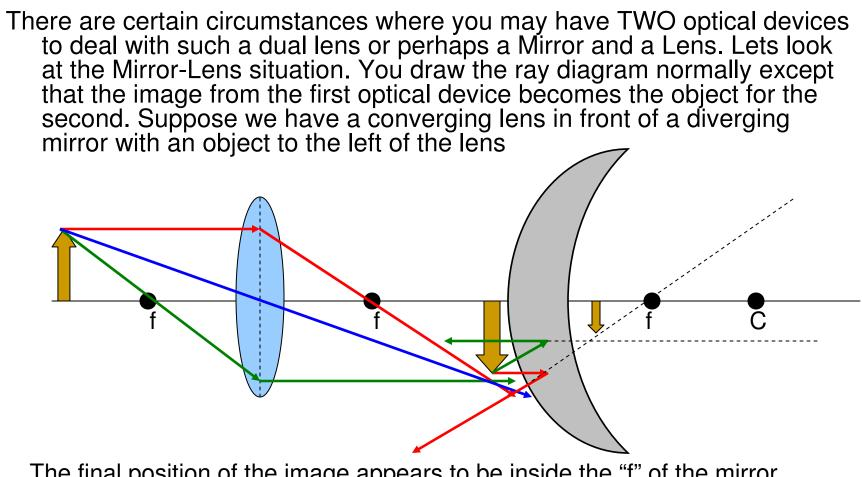
The final position of the image appears to be inside the "f" of the mirror, VIRTUAL, REDUCED and INVERTED. We really need to apply the optics equations to verify our picture.
