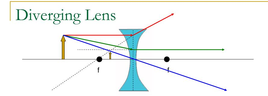
The image is VIRTUAL, REDUCED, and UPRIGHT. On the next slide we will verify with the math. But before we do it is important to understand that all DIVERGING LENSES AND MIRRORS have **NEGATIVE FOCAL** LENGTHS!!!.
