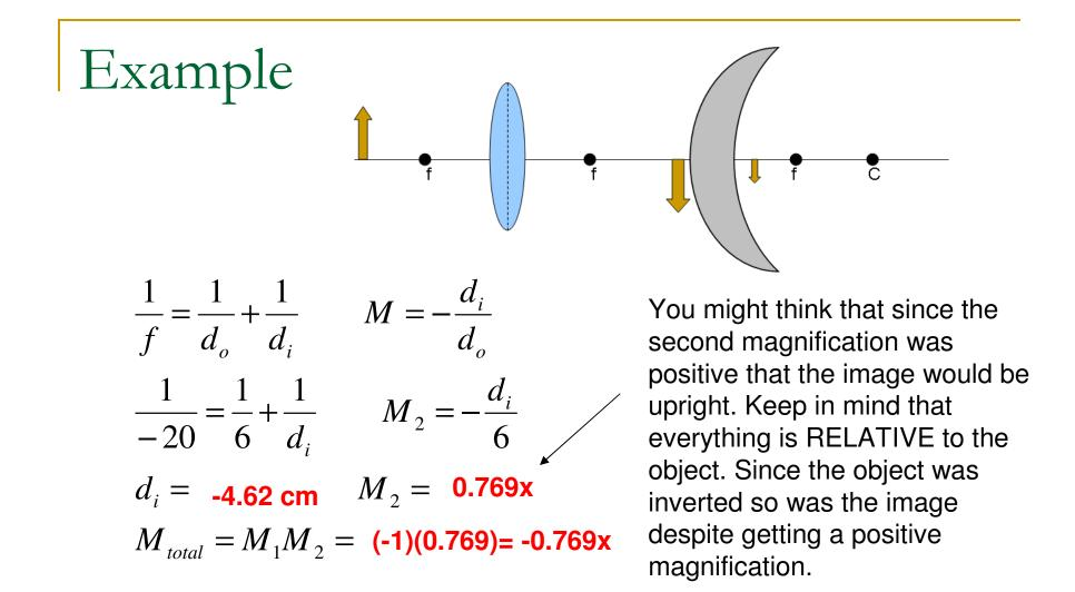
So the FINAL image is VIRTUAL, INVERTED, and REDUCED..relative to the original object.
