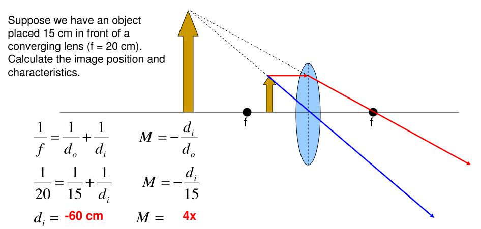
As we thought. The image distance is negative, thus making it a VIRTUAL image. The magnification was positive and greater than 1, making it enlarged and upright. This is a MAGNIFYING GLASS!
